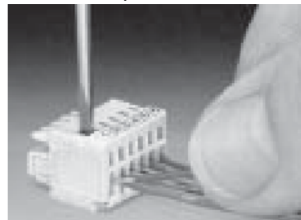
Image 2.22 Fitting the cable to the connector
