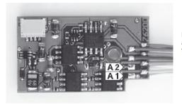
Located on the top side of the decoder, right beside the notch are the solder pads for A1 and A2 for connection of the special functions.
