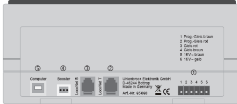
Figure 3.11 The rear of the IB-COM showing the connections
